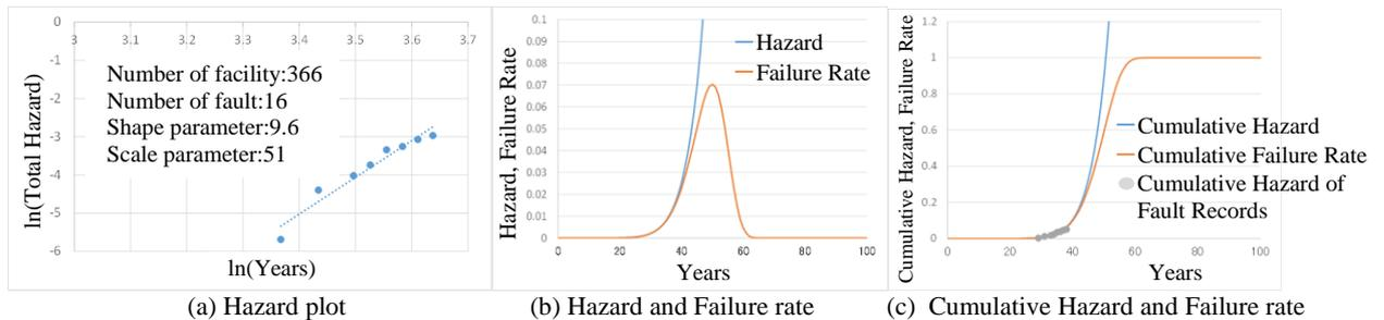
**Figure 2 Fault analysis of vacuum circuit breaker of 6 kV switchgear**
